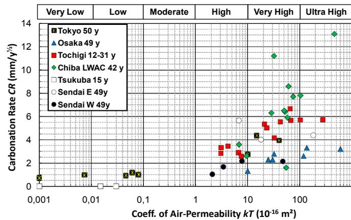
Figure 3.  $CR$  and  $kT$  values measured on Japanese Structures
