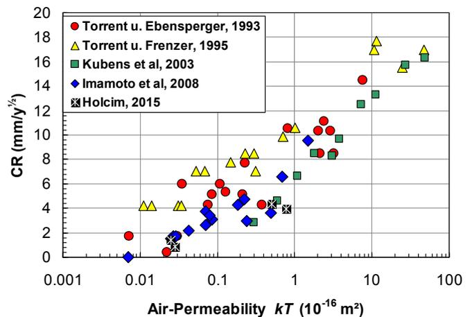
Figure 1.  $CR$  measured in the lab under natural  $CO_2$  exposure vs.  $kT$  values
