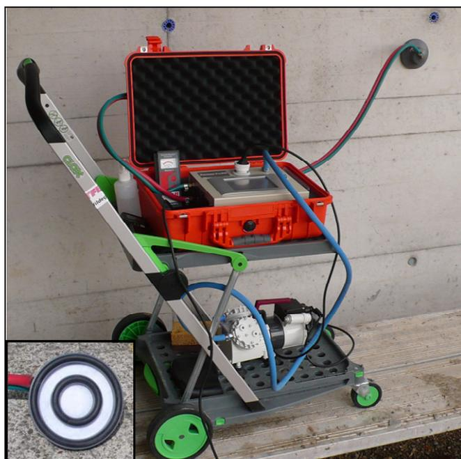
Figure 9.  $kT$  test: details of vacuum cell and application on a concrete wall
