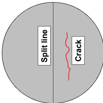
Figure 6. Possible crack affecting  $kT$  but not  $CD$  measured on the core split surface
