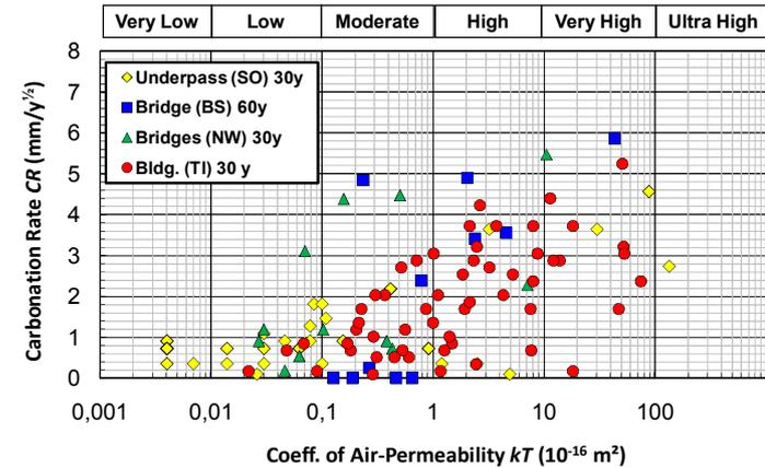
Figure 2.  $CR$  and  $kT$  values measured on Swiss Structures
