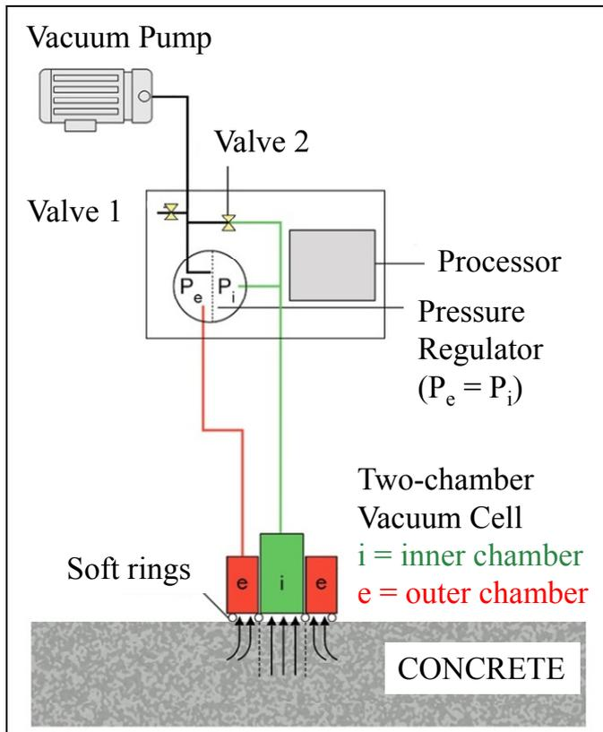
Figure 8. Sketch of  $kT$  test [SIA 262/1, 2013]
